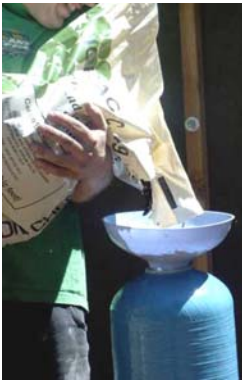
Adding media to the tank.
